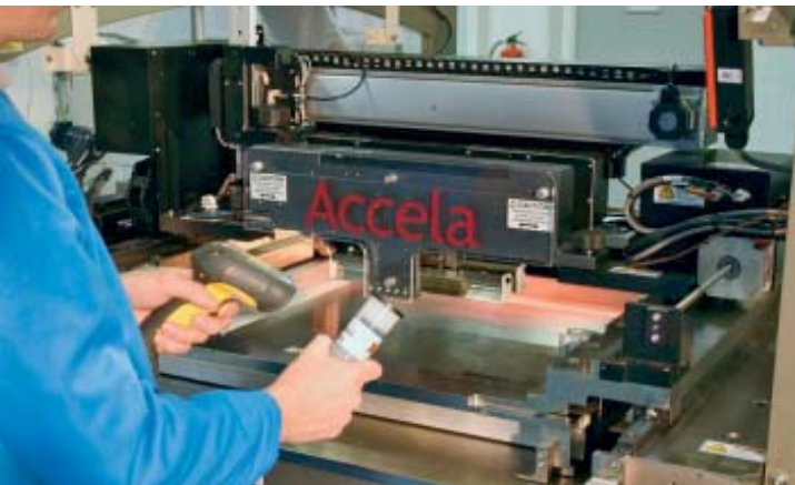
Data acquisition of paste cartridge with external barcode scanner
