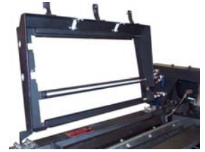
Nitrogen shroud in service position
